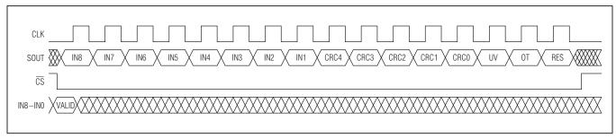
Figure 4. SPI Communication Example
