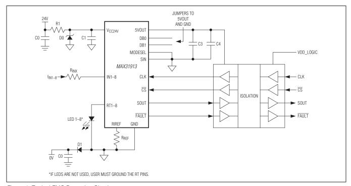
Figure 1. Typical EMC Protection Circuitry
