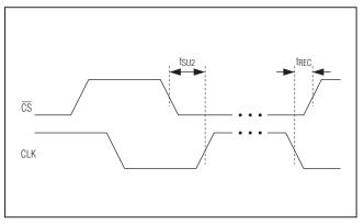
Figure 6. SPI Timing Diagram 2
