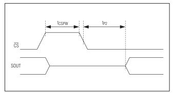
Figure 5. SPI Timing Diagram 1
