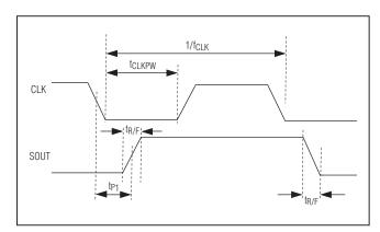
Figure 8. SPI Timing Diagram 4
