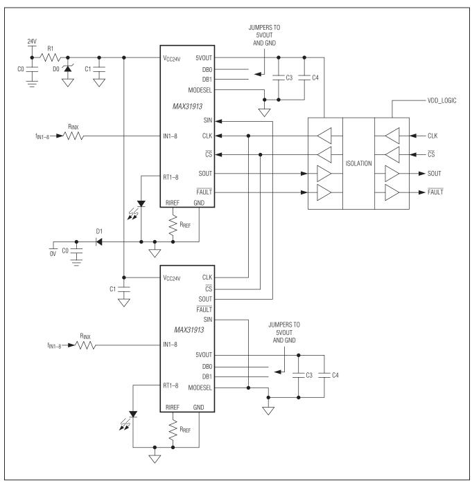
Figure 3. 16-Input Application Circuit
